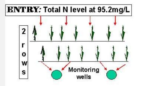
EXIT: Total N level at 16mg/L or a reduction of 83%
