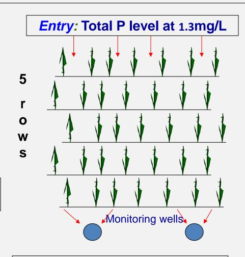
Exit: Total P level at 0.20mg/L or a reduction of 85%
