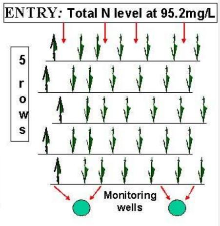
EXIT Total N level at 1.2mg/L or a reduction of 99%
