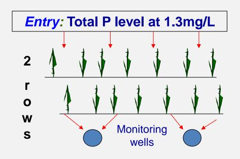
Exit: Total P level at 0.24mg/L or a reduction of 82%
